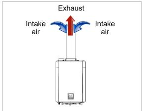
Figure 15: Concentric Pipe
