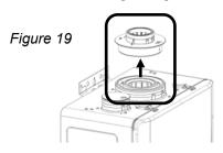
3. Install the concentric vent. Ensure it is properly seated.
