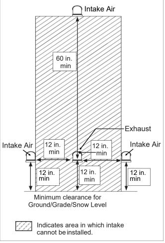
Figure 25: Horizontal Vent and Intake Air Piping
