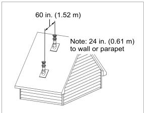
Figure 16: Between terminals at different levels
