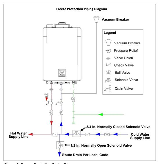
Figure 6: Freeze Protection Piping Diagram
