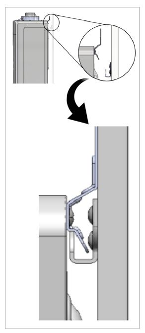
Figure 10: Mount the top bracket
