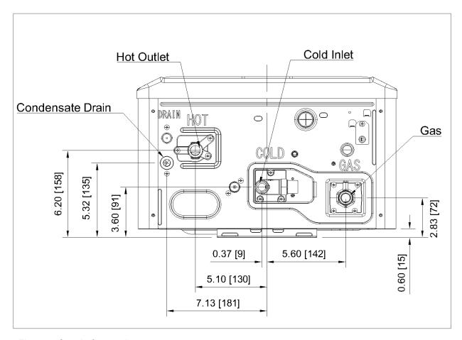
Figure 5: Supply Connections
