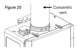
4. Secure the vent pipe to the concentric flue connection with the supplied screws.
