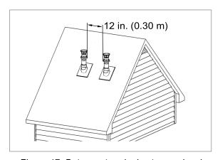
Figure 17: Between terminals at same level
