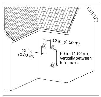
Figure 14: Concentric Pipe Termination Clearances
