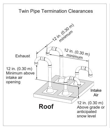
Figure 24: Twin Pipe Vertical Termination of Multiple Water Heaters
